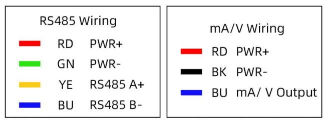
XNote: When wiring, connect the positive and negative poles of the power supply first, and then connect the signal wire
