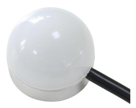
KM75B61 using the standard RS485 bus MODBUS-RTU protocol, easy access to PLC, DCS and other instruments or systems for monitoring illuminance state quantities. The internal use of high-precision sensing core and related devices to ensure high reliability and excellent long-term stability, can be customized RS232, RS485, CAN, 4-20mA, DC0~5V\10V, ZIGBEE, Lora, WIFI, GPRS and other output methods.
