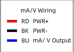
Note: When wiring, connect the positive and negative poles
