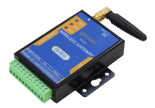
QM5095B using the standard USB, easy access to PLC, DCS and other instruments or systems for monitoring RS485 state quantities. The internal use of high-precision sensing core and related devices to ensure high reliability and excellent long-term stability, can be customized
