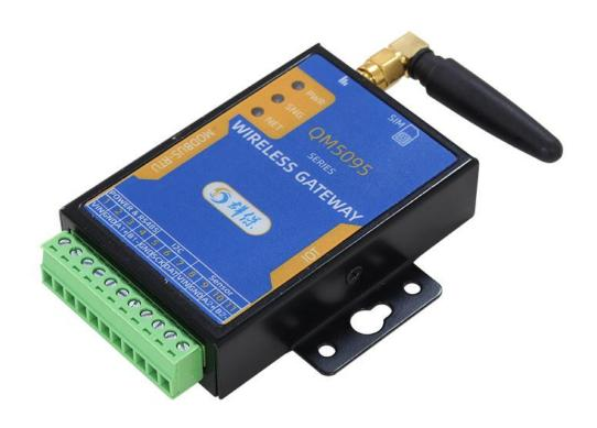
QM5095I using the standard USB, easy access to PLC, DCS and other instruments or systems for monitoring I2C state quantities. The internal use of high-precision sensing core and related devices to ensure high reliability and excellent long-term stability, can be customized RS232,RS485,CAN,4-20mA,DC0~5V\10V,ZIGBEE,Lora,WIFI,GPRS and other output methods.
