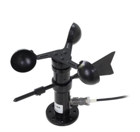
INTEGRATED SENSOR FOR WIND SPEED AND DIRECTION (EXCLUDING ANY OTHER ACCESSORIES)
