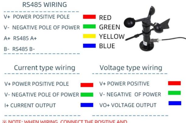
※ NOTE: WHEN WIRING, CONNECT THE POSITIVE AND NEGATIVE POLE OF THE POWER SUPPLY FIRST, AND THEN CONNECT THE SIGNAL WIRE
