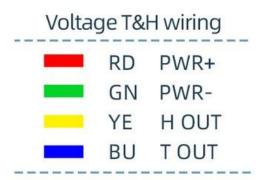
※Note: When wiring, first connect the positive and negative
