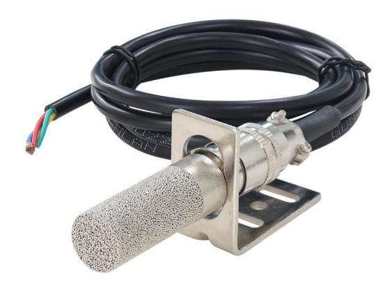
QM7820B using the standard RS485 bus MODBUS-RTU protocol, easy access to PLC, DCS and other instruments or systems for monitoring temperature, humidity state quantities. The internal use of high-precision sensing core and related devices to ensure high reliability and excellent long-term stability, can be customized RS232, RS485, CAN, 4-20mA, DC0~5V\10V, ZIGBEE, Lora, WIFI, GPRS and other output methods.
