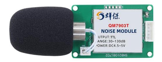
QM7903T using the standard ,easy access to PLC. DCS and other instruments or systems for monitoring noise state quantities. The internal use of high-precision sensing core and related devices to ensure high reliability and excellent long-term stability, can be customized RS232,RS485,CAN,4-20mA,DC0~5V\10V,ZIGBEE,Lora,WIFI,GPRS and other output methods.
