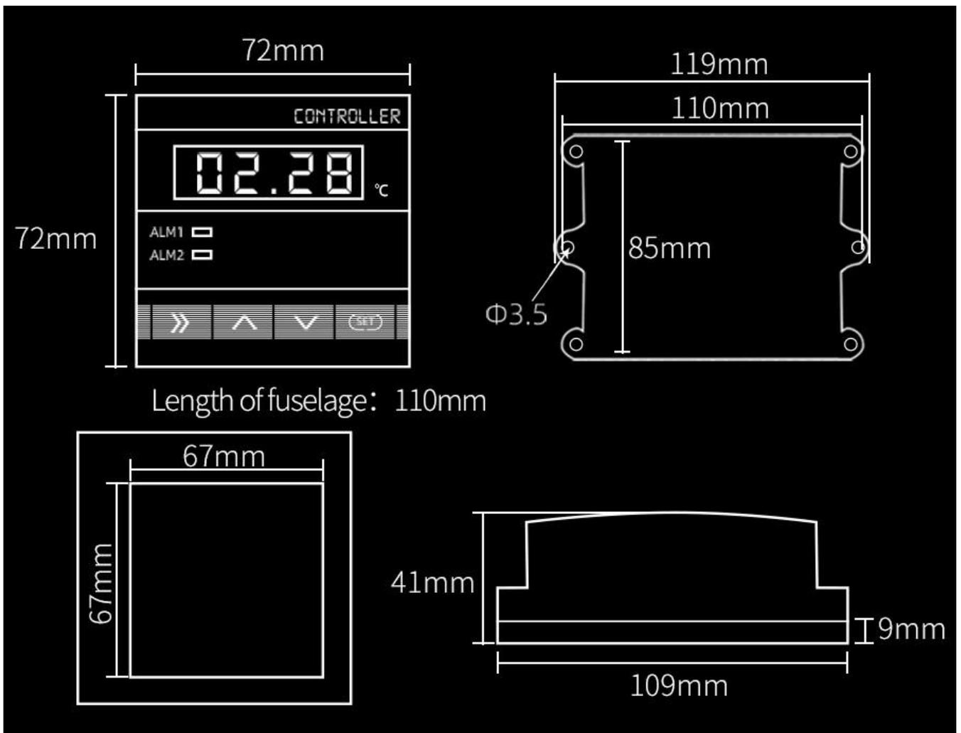
Length of fuselage: 110mm
