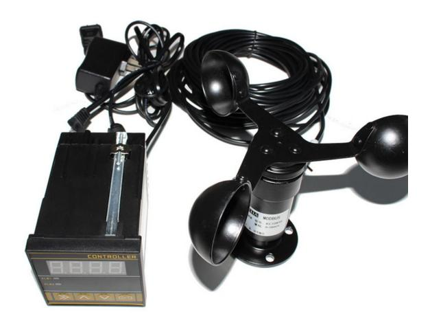
SC7239 using the standard RS485 bus MODBUS-RTU protocol, easy access to PLC, DCS and other instruments or systems for monitoring wind speed state quantities. The internal use of high-precision sensing core and related devices to ensure high reliability and excellent long-term stability, can be customized RS232, RS485, CAN, 4-20mA, DC0~5V\10V, ZIGBEE, Lora, WIFI, GPRS and other output methods.
