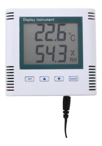
SD6711B using the standard RS485 bus MODBUS-RTU protocol, easy access to PLC, DCS and other instruments or systems for monitoring 0~100%RH state quantities. The internal use of high-precision sensing core and related devices to ensure high reliability and excellent long-term stability, can be customized RS232,RS485,CAN,4-20mA,DC0~5V\10V,ZIGBEE,Lora,WIFI,GPRS and other output methods.
