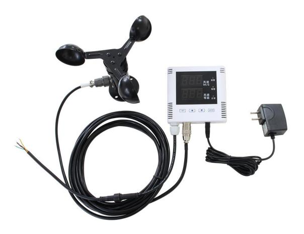
SD6786B using the standard RS485 bus MODBUS-RTU protocol, easy access to PLC, DCS and other instruments or systems for monitoring wind speed state quantities. The internal use of high-precision sensing core and related devices to ensure high reliability and excellent long-term stability, can be customized RS232, RS485, CAN, 4-20mA, DC0~5V\10V, ZIGBEE, Lora, WIFI, GPRS and other output methods.
