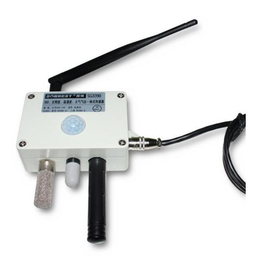
SG3390 using the standard RS485 bus MODBUS-RTU protocol, easy access to PLC, DCS and other instruments or systems for monitoring humidity state quantities. The internal use of high-precision sensing core and related devices to ensure high reliability and excellent long-term stability, can be customized RS232,RS485,CAN,4-20mA,DC0~5V\10V,ZIGBEE,Lora,WIFI,GPRS and other output methods.
