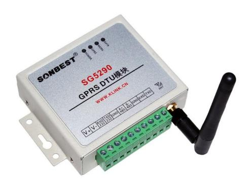
SG5290 using the standard GPRS Wireless Interface, easy access to PLC. DCS and other instruments or systems for monitoring RS485 state quantities. The internal use of high-precision sensing core and related devices to ensure high reliability and excellent long-term stability, can be customized RS232,RS485,CAN,4-20mA,DC0~5V\10V,ZIGBEE,Lora,WIFI,GPRS and other output methods.
