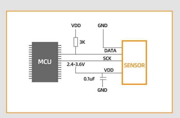
THE PRODUCT FUNCTION AND USAGE METHOD ARE CONSISTENT WITH SHT20 OR SHT30 CHIPS. NEEDIT CAN ONLY BE USED BY PROGRAMMING OR CONNECTING THE CORRESPONDING MODULE
