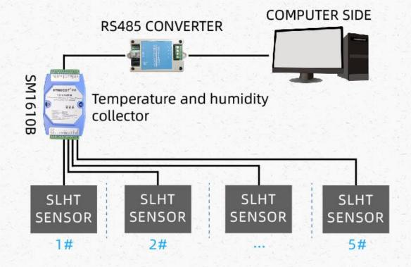
Use scheme with temperature and humidity module
