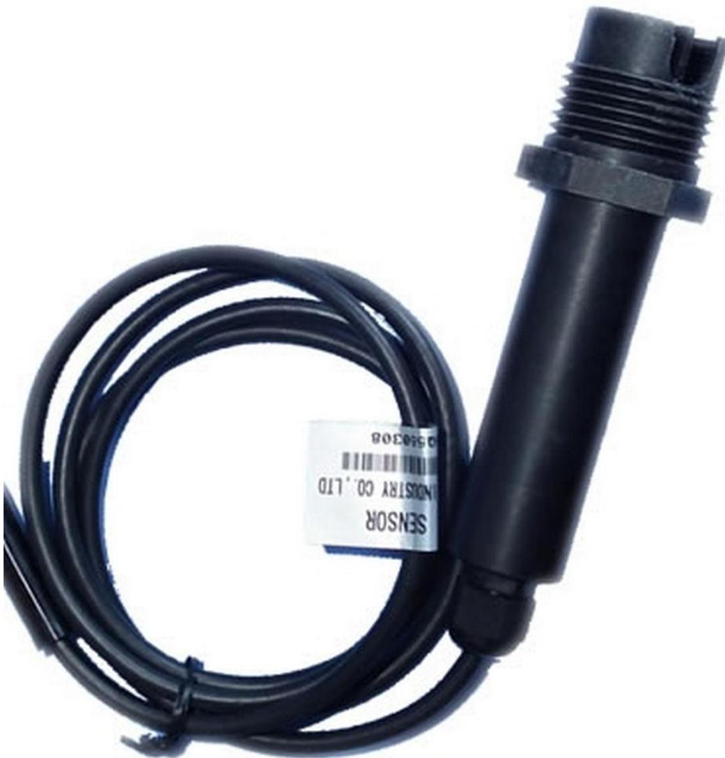
SLP2000 using the standard DC4-20mA current output signal, easy access to PLC, DCS and other instruments or systems for monitoring salinity state quantities. The internal use of high-precision sensing core and related devices to ensure high reliability and excellent long-term stability, can be customized RS232, RS485, CAN, 4-20mA, DC0~5V/10V, ZIGBEE, Lora, WIFI, GPRS and other output methods.
