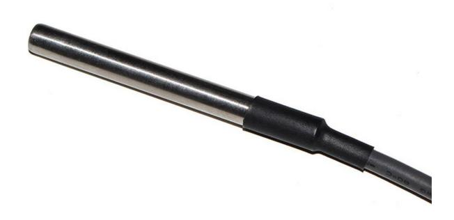
SLST1 series digital temperature sensor adopts DS18B20 digital temperature sensor from Dallas Semiconductor of the United States. The sensor is packaged in a stainless steel case and is waterproof and moisture-proof. The specially designed sensor stainless steel case has a wall thickness of only
