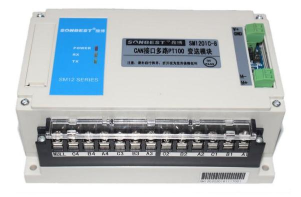
SM1201C using the standard CAN Bus, easy access to PLC, DCS and other instruments or systems for monitoring temperature @8 state quantities. The internal use of high-precision sensing core and related devices to ensure high reliability and excellent long-term stability, can be customized RS232,RS485,CAN,4-20mA,DC0~5V\10V,ZIGBEE,Lora,WIFI,GPRS and other output methods.
