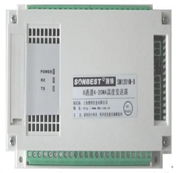
SM1201M using the standard DC4-20mA current output signal, easy access to PLC, DCS and other instruments or systems for monitoring temperature @12 state quantities. The internal use of high-precision sensing core and related devices to ensure high reliability and excellent long-term stability, can be
