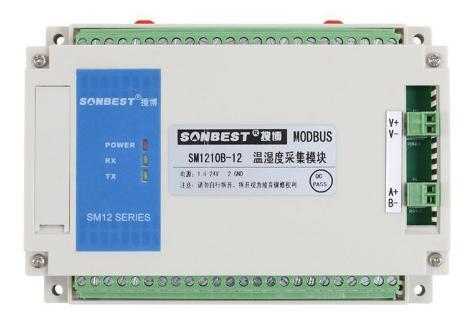
SM1210B-12 using the standard RS485 bus MODBUS-RTU protocol, easy access to PLC, DCS and other instruments or systems for monitoring temperature, humidity@12 state quantities. The internal use of high-precision sensing core and related devices to ensure high reliability and excellent long-term
