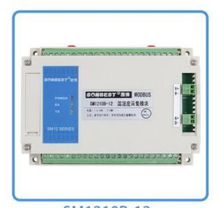
SM1210B-12 Temperature and humidity acquisition module
