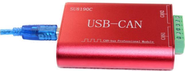
The product uses the CAN2.0B standard frame format. The standard frame information is 11 bytes, including two parts of information and the first 3 bytes of the data part are the information part. The default node number is 1 when the device leaves the factory, which means The text identification code is ID.10-ID.3 in the CAN standard frame, and the default rate is 50k. If other rates are required, they can be modified according to the communication protocol.
