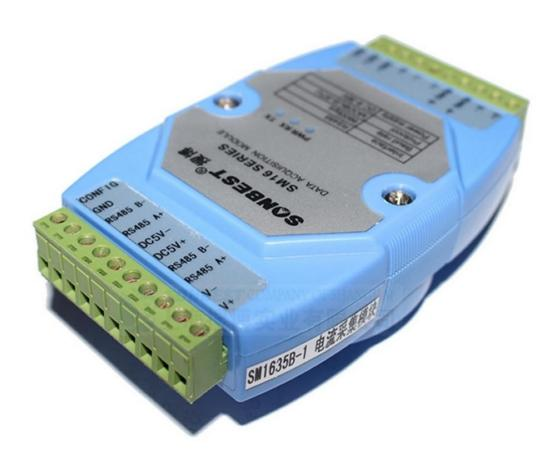
SM1601B using the standard RS485 bus MODBUS-RTU protocol, easy access to PLC, DCS and other instruments or systems for monitoring temperature state quantities. The internal use of high-precision sensing core and related devices to ensure high reliability and excellent long-term stability, can be customized RS232,RS485,CAN,4-20mA,DC0~5V\10V,ZIGBEE,Lora,WIFI,GPRS and other output methods.
