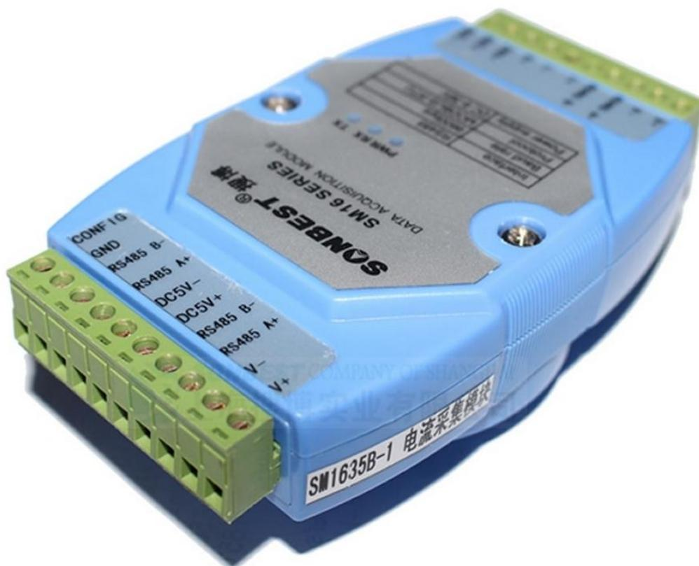
SM1602B using the standard RS485 bus MODBUS-RTU protocol, easy access to PLC, DCS and other instruments or systems for monitoring temperature state quantities. The internal use of high-precision sensing core and related devices to ensure high reliability and excellent long-term stability, can be customized RS232, RS485, CAN, 4-20mA, DC0~5V\10V, ZIGBEE, Lora, WIFI, GPRS and other output methods.
