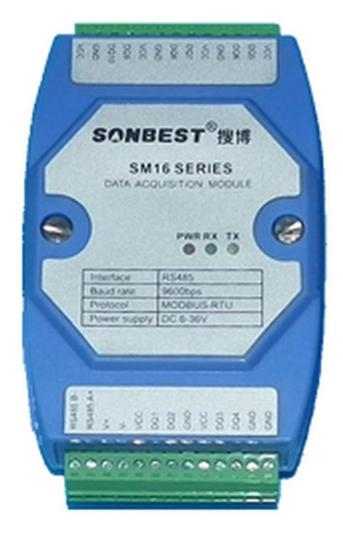
SM1633B-8 using the standard RS485 bus MODBUS-RTU protocol, easy access to PLC, DCS and other instruments or systems for monitoring 4-20MAcurrent state quantities. The internal use of high-precision sensing core and related devices to ensure high reliability and excellent long-term stability, can be customized RS232, RS485, CAN, 4-20mA, DC0~5V\10V, ZIGBEE, Lora, WIFI, GPRS and other output methods.
