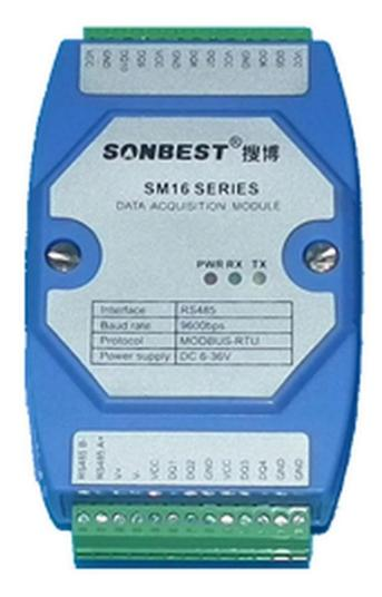
SM1650B-8 using the standard RS485 bus MODBUS-RTU protocol,easy access to PLC,DCS and other instruments or systems for monitoring 开关量 state quantities. The internal use of high-precision sensing core and related devices to ensure high reliability and excellent long-term stability, can be customized RS232,RS485,CAN,4-20mA,DC0~5V\10V,ZIGBEE,Lora,WIFI,GPRS and other output methods.
