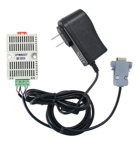
SM1800A using the standard ,easy access to PLC, DCS and other instruments or systems for monitoring temperature state quantities. The internal use of high-precision sensing core and related devices to ensure high reliability and excellent long-term stability, can be customized
