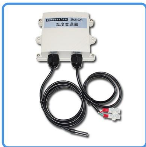
Protected 4-20mA temperature PT1000 current transmitter
