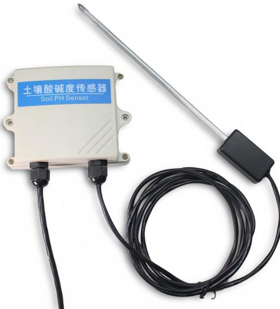
SM2120M using the standard DC4-20mA current output signal,easy access to PLC, DCS and other instruments or systems for monitoring soil pH state quantities.The internal use of high -precision sensing core and related devices to ensure high reliability and excellent long-term stability,can be customized RS232,RS485,CAN,4-20mA,DC0~5V\10V,ZIGBEE,Lora,WIFI,GPRS and other output methods.
