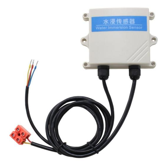
SM2138B using the standard RS485 bus MODBUS-RTU protocol, easy access to PLC, DCS and other instruments or systems for monitoring flooding state quantities. The internal use of high-precision sensing core and related devices to ensure high reliability and excellent long-term stability, can be customized RS232, RS485, CAN, 4-20mA, DC0~5V\10V, ZIGBEE, Lora, WIFI, GPRS and other output methods.
