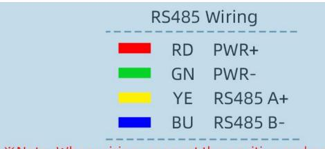
XNote: When wiring, connect the positive and negative poles of the power supply first, and then connect the signal wire
