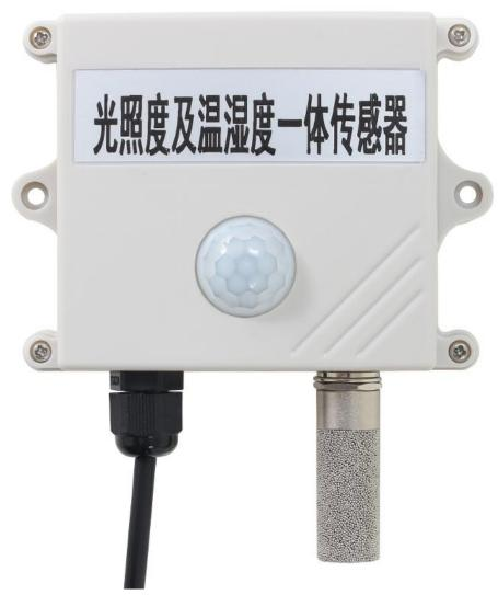
SM2190B using the standard RS485 bus MODBUS-RTU protocol, easy access to PLC, DCS and other instruments or systems for monitoring illuminance, temperature, humidity state quantities. The internal use of high-precision sensing core and related devices to ensure high reliability and excellent long-term stability, can be customized RS232, RS485, CAN, 4-20mA, DC0~5V\10V, ZIGBEE, Lora, WIFI, GPRS and other output methods.
