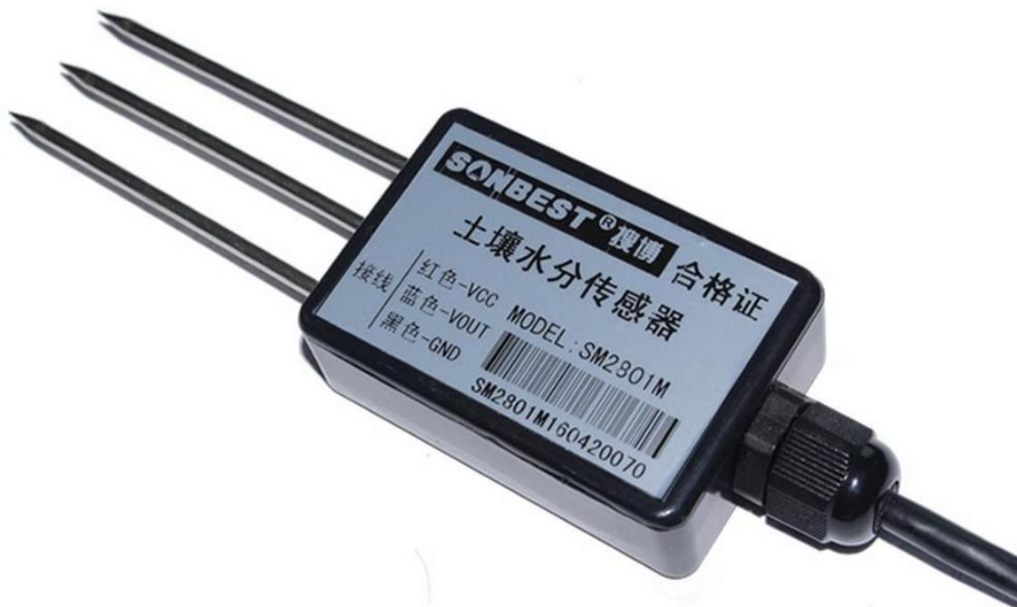
SM2801M using the standard DC4-20mA current output signal, easy access to PLC, DCS and other instruments or systems for monitoring 24% soil Moisture state quantities. The internal use of high-precision sensing core and related devices to ensure high reliability and excellent long-term stability, can be customized RS232, RS485, CAN, 4-20mA, DC0~5V\10V, ZIGBEE, Lora, WIFI, GPRS and other output methods.
