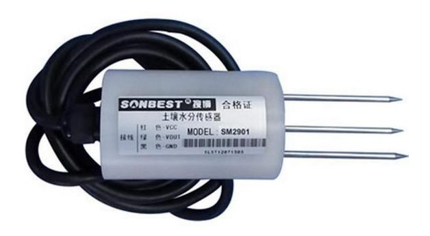
SM2901M using the standard DC4-20mA current output signal, easy access to PLC. DCS and other instruments or systems for monitoring 24%soil Moisture state quantities. The internal use of high-precision sensing core and related devices to ensure high reliability and excellent long-term stability, can be customized RS232, RS485, CAN, 4-20mA, DC0~5V\10V, ZIGBEE, Lora, WIFI, GPRS and other output methods.
