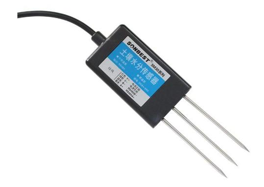
SM3102B using the standard RS485 bus MODBUS-RTU protocol, easy access to PLC, DCS and other instruments or systems for monitoring soil Moisture, soil temperature state quantities. The internal use of high-precision sensing core and related devices to ensure high reliability and excellent long-term stability, can be customized RS232, RS485, CAN, 4-20mA, DC0~5V\10V, ZIGBEE, Lora, WIFI, GPRS and other output methods.
