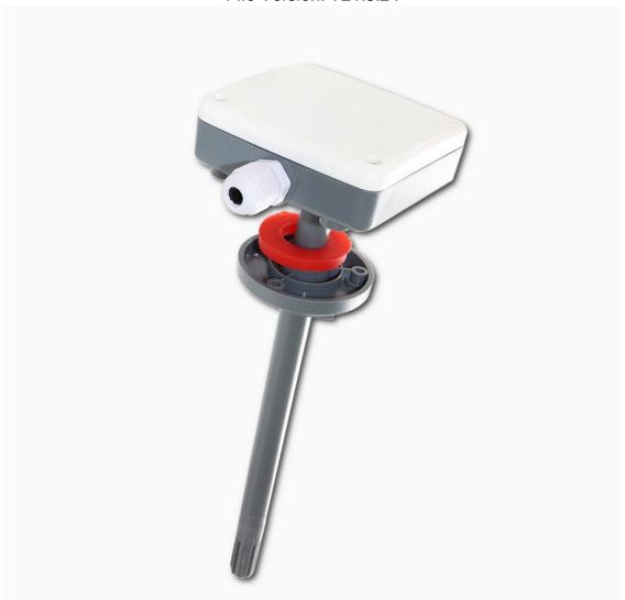
SM3710V using the standard DC0 ~ 10V voltage output signal,easy access to PLC. DCS and other instruments or systems for monitoring temperature, humidity state quantities. The internal use of high-precision sensing core and related devices to ensure high reliability and excellent long-term stability, can be customized RS232, RS485, CAN, 4-20mA, DC0~5V\10V, ZIGBEE, Lora, WIFI, GPRS and other output methods.
