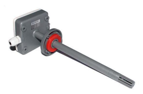
SM3710V2 using the standard DC0 ~ 10V voltage output signal,easy access to PLC, DCS and other instruments or systems for monitoring temperature,humidity state quantities. The internal use of high-precision sensing core and related devices to ensure high reliability and excellent long-term stability,can be customized RS232,RS485,CAN,4-20mA,DC0~5V\10V,ZIGBEE,Lora,WIFI,GPRS and other output methods.
