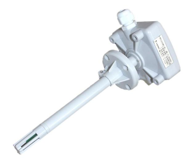
SM3810V using the standard DC0 ~ 10V voltage output signal,easy access to PLC, DCS and other instruments or systems for monitoring temperature,humidity state quantities. The internal use of high-precision sensing core and related devices to ensure high reliability and excellent long-term stability,can be customized RS232,RS485,CAN,4-20mA,DC0~5V\10V,ZIGBEE,Lora,WIFI,GPRS and other output methods.
