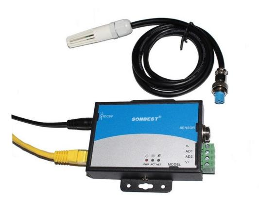
SM5010T using the standard TCP/IP Network Interface, easy access to PLC, DCS and other instruments or systems for monitoring temperature, humidity state quantities. The internal use of high-precision sensing core and related devices to ensure high reliability and excellent long-term stability, can be customized RS232, RS485, CAN, 4-20mA, DC0~5V\10V, ZIGBEE, Lora, WIFI, GPRS and other output methods.
