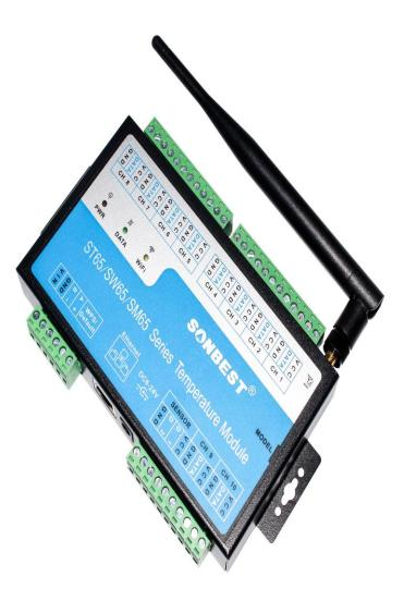
SM6500T using the standard RS485 bus MODBUS-RTU protocol, easy access to PLC, DCS and other instruments or systems for monitoring temperature@10 state quantities. The internal use of high-precision sensing core and related devices to ensure high reliability and excellent long-term stability, can be customized RS232, RS485, CAN, 4-20mA, DC0~5V\10V, ZIGBEE, Lora, WIFI, GPRS and other output methods.
