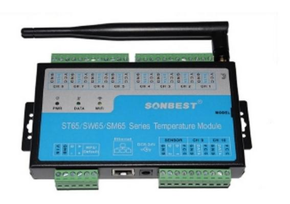
SM6501T using the standard TCP/IP Network Interface, easy access to PLC, DCS and other instruments or systems for monitoring temperature state quantities. The internal use of high-precision sensing core and related devices to ensure high reliability and excellent long-term stability, can be customized RS232,RS485,CAN,4-20mA,DC0~5V\10V,ZIGBEE,Lora,WIFI,GPRS and other output methods.
