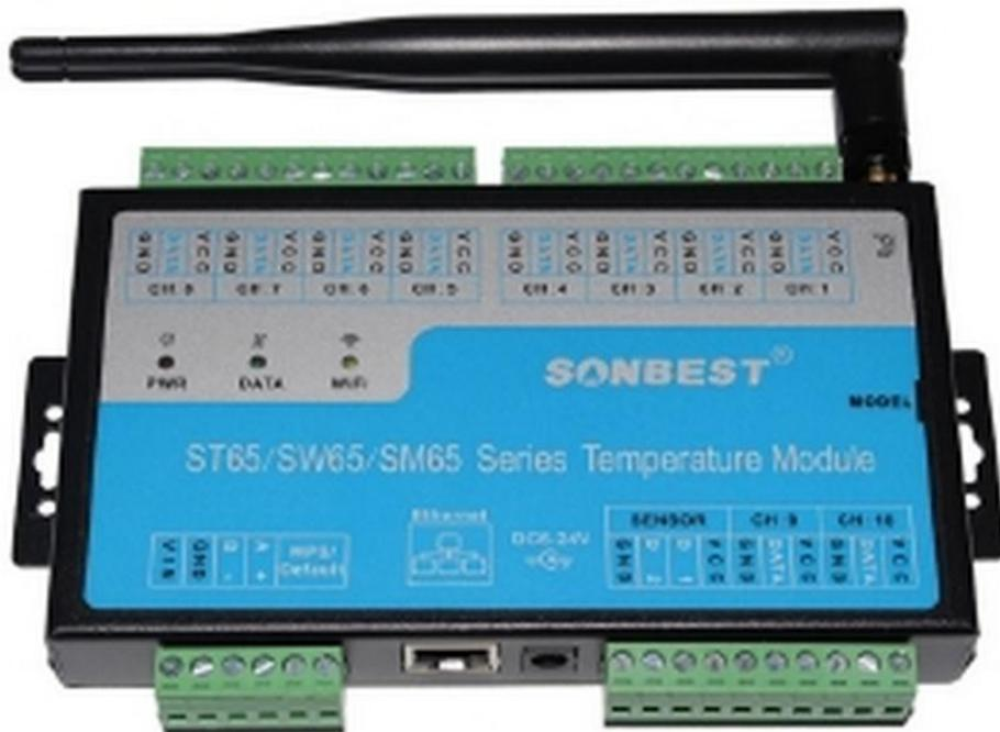
SM6510T using the standard TCP/IP Network Interface, easy access to PLC, DCS and other instruments or systems for monitoring temperature, humidity state quantities. The internal use of high-precision sensing core and related devices to ensure high reliability and excellent long-term stability, can be customized RS232, RS485, CAN, 4-20mA, DC0~5V/10V, ZIGBEE, Lora, WIFI, GPRS and other output methods.
