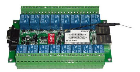
SM6516T using the standard TCP/IP Network Interface, easy access to PLC, DCS and other instruments or systems for monitoring state quantities. The internal use of high-precision sensing core and related devices to ensure high reliability and excellent long-term stability, can be customized RS232,RS485,CAN,4-20mA,DC0~5V\10V,ZIGBEE,Lora,WIFI,GPRS and other output methods.
