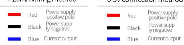
In the case of broken wires, wire the wires as shown in the figure. If the product itself has no leads, the core color is for reference.
