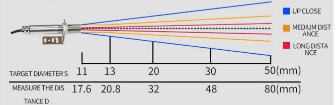
D: S IS THE OPTICAL RESOLUTION, REPRESENTING THE RATIO OF THE DIAMETER OF THE SPOT AT THE DISTANCE TO THE MEASUREMENT PO INT SUCH AS THE FOREHEAD DIAMETER OF ABOUT 30 MM FOR A DISTANCE MEASUREMENT OF 480 MM FOR A DISTANCE MEASUREMENT OF UP TO 48 MM FOR A DISTANCE MEASUREMENT OF UP TO 36 MM FOR A CL OSE MEASUREMENT
