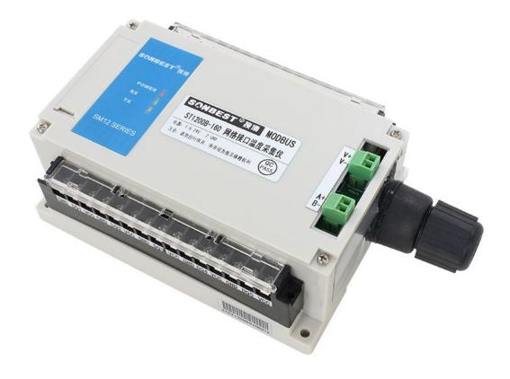
ST1200B using the standard TCP/IP Network Interface, easy access to PLC, DCS and other instruments or systems for monitoring temperaturex=100@10 state quantities. The internal use of high-precision sensing core and related devices to ensure high reliability and excellent long-term
