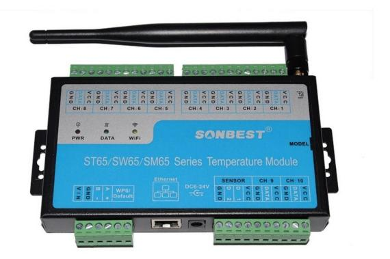
SW6500T using the standard Wireless Interface, easy access to PLC, DCS and other instruments or systems for monitoring temperature state quantities. The internal use of high-precision sensing core and related devices to ensure high reliability and excellent long-term stability, can be customized RS232, RS485, CAN, 4-20mA, DC0~5V\10V, ZIGBEE, Lora, WIFI, GPRS and other output methods.
