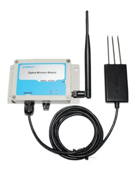
SZ2030C using the standard ZIGBEE Wireless Communication Interface, easy access to PLC, DCS and other instruments or systems for monitoring soil Moisture state quantities. The internal use of high-precision sensing core and related devices to ensure high reliability and excellent long-term stability, can be customized RS232, RS485, CAN, 4-20mA, DC0~5V\10V, ZIGBEE, Lora, WIFI, GPRS and other output methods.
