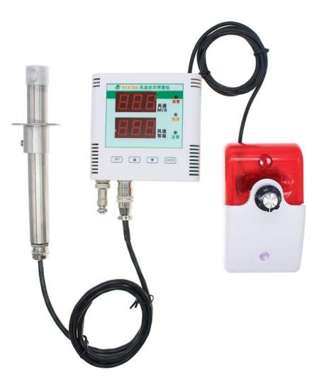
XD6789 using the standard RS485 bus MODBUS-RTU protocol, easy access to PLC, DCS and other instruments or systems for monitoring wind speed state quantities. The internal use of high-precision sensing core and related devices to ensure high reliability and excellent long-term stability, can be customized RS232,RS485,CAN,4-20mA,DC0~5V\10V,ZIGBEE,Lora,WIFI,GPRS and other output methods.
