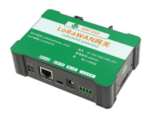
XM1302 using the standard ,easy access to PLC. DCS and other instruments or systems for monitoring LORA state quantities. The internal use of high-precision sensing core and related devices to ensure high reliability and excellent long-term stability, can be customized RS232,RS485,CAN,4-20mA,DC0~5V\10V,ZIGBEE,Lora,WIFI,GPRS and other output methods.
