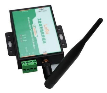
XM5090 using the standard RS485 bus MODBUS-RTU protocol, easy access to PLC, DCS and other instruments or systems for monitoring LORA state quantities. The internal use of high-precision sensing core and related devices to ensure high reliability and excellent long-term stability, can be customized RS232,RS485,CAN,4-20mA,DC0~5V\10V,ZIGBEE,Lora,WIFI,GPRS and other output methods.
